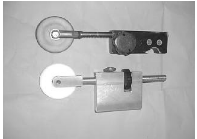
A good example of reverse engineering to improve a headache. The original OEM product continually failed and needed to be replaced, plus it lacked adjustability. Sabattus redesigned the part, included a fine adjustment feature and now the part will last for years.
